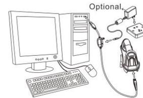
1. Please charge the battery before the first time of use. The charge indicator on the handheld unit is turned on when the charging is in process. When the charging process completes, the charge indicator is turned off.
